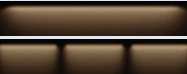
LED Linear lighting (top) creates smooth lighting effect with no socket shadows, where as fluorescent lighting (bottom) creates socket shadows between tubes. (For illustrative purposes only. Image based on three fixtures placed end to end.)
